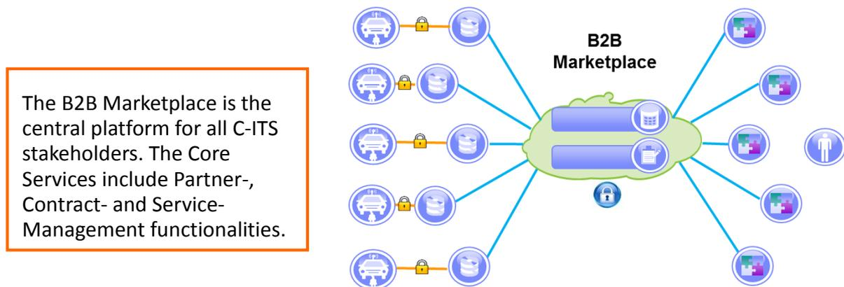
The B2B marketplace features a kind of additional layer between the vehicle and the service providers, which would be fed by vehicle manufacturers' back end servers. An association consisting of all C-ITS stakeholders is also required to control the marketplace, and one of the objectives is notably to solve the monitoring issue thanks to end-to-end encryption.
