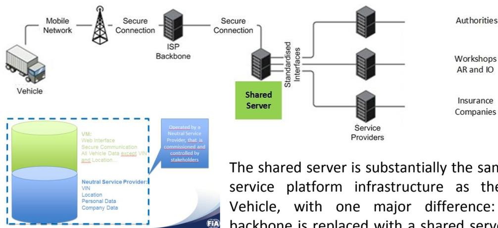
The shared server is substantially the same technical service platform infrastructure as the Extended Vehicle, with one major difference: the OEM backbone is replaced with a shared server operated by a neutral service provider commissioned and controlled by a consortium representing interested stakeholders. This shared server would control at least personal and business data, other data remaining under the control of vehicle manufacturers.
