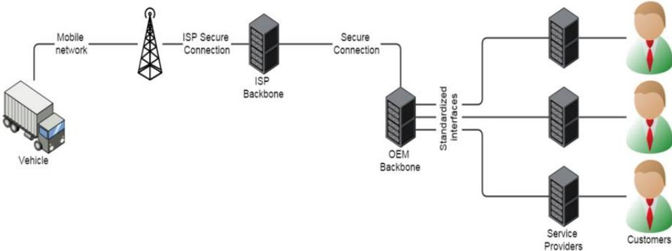
With the data server of the Extended Vehicle, the data are transferred via the mobile telecom networks from the vehicle to the vehicle manufacturer's server (OEM backbone), and then made accessible to service providers via a standardised interface. Data types are linked to use cases, each use case can be a specific standardisation item. Independent operators and service providers pointed out that this does not sufficiently address the access conditions (time criticality, B2B contracts etc.).
