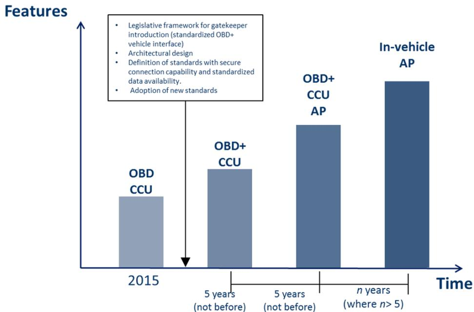
The figure above summarises this evolutionary approach, which underlines (see the box in the figure) the necessity to have a legislative framework for gatekeeper introduction (OBD+ vehicle interface), and the definition of necessary standards for the OBD+ interface, secure connection capability and standardised data availability, to see this evolution happen concretely.
